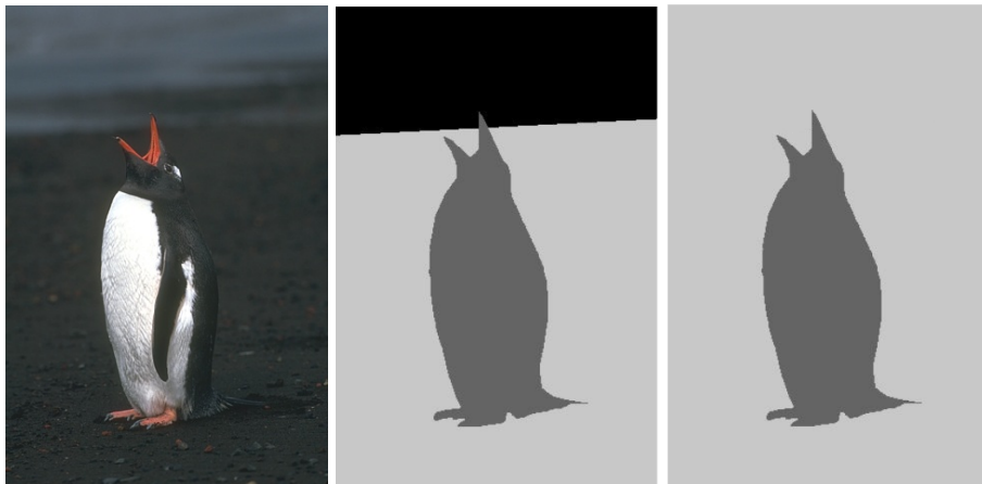
Fig. 4. Original image, ground truth, and a possible segmentation produced by an algorithm for an image from the Berkeley dataset.
